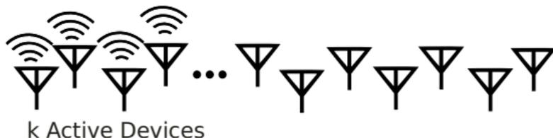
**Phase 3 (Uplink Payload Transmission):** The  $k$  active users transmit their payload in the  $k$  slots based on the schedule provided by the BS, while avoiding collision.
